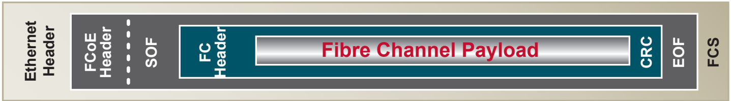
Figure 3. In FCoE, the Fibre Channel payload is encapsulated in Ethernet frames.
